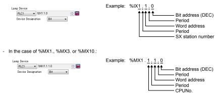
\*3 Double-word addresses (%MD1., %MD3. or %MD10.) can be set for PLC1 only. To enable access to these addresses from PLC2 to PLC8, use a word address (%MW1., %MW3. or %MW10.) and set two words for data length. Example: To access the %MD1.100 address, use %MW1.100, and set two words for data length.
