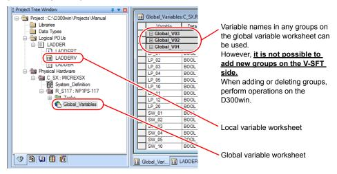
\* The characters used for variable names are limited. For details, refer to the next section and the MICREX-SX User's Manual <Instructions> (FEH200).
