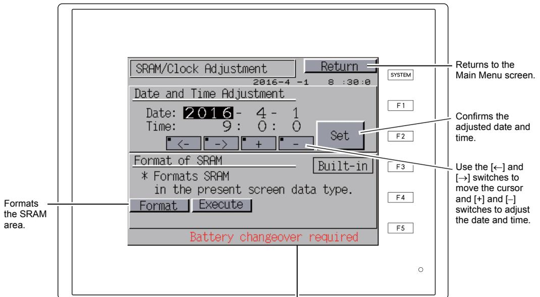
A "Battery changeover required" alert message is displayed here <sup>\*1</sup>.
